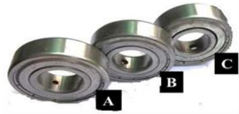
Fig.4 Tests bearings with IRF
